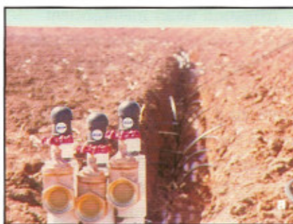
Figure 7. Laying subsurface drip (a) and the pump that maintains the flow of water through the system (b).
