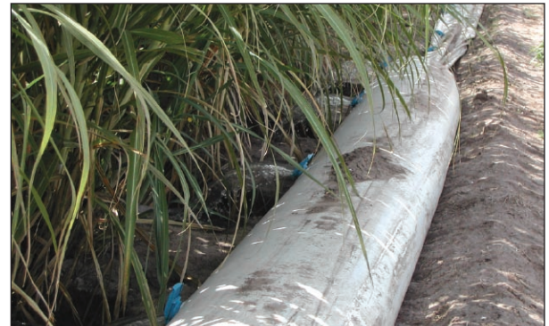
Figure 8b. Gate holes used to irrigate sugarcane.
