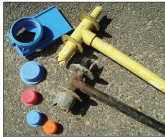
Figure 6. Hole puncher, plugs, and gates for poly-pipe.
